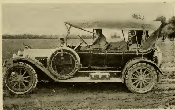
On the dirt roads of the Middle West prairie States it is a wise precaution to use Weed chains on front and rear wheels when the roads are wet
